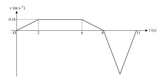
The diagram shows the velocity-time graph for the motion of a machine's cutting tool. The graph consists of five straight line segments. The tool moves forward for 8 s while cutting and then takes 3 s to return to its starting position. Find
