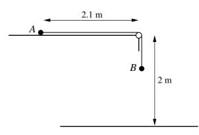
Particles A and B, of masses 0.2 kg and 0.45 kg respectively, are connected by a light inextensible string of length 2.8 m. The string passes over a small smooth pulley at the edge of a rough horizontal surface, which is 2 m above the floor. Particle A is held in contact with the surface at a distance of 2.1 m from the pulley and particle B hangs freely (see diagram). The coefficient of friction between A and the surface is 0.3. Particle A is released and the system begins to move.
